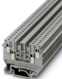
1-level terminal block with double connection on both sides, cross section: 0.2 - 2.5 mm 2 , AWG: 24 - 10, width: 6.2 mm, color: blue
