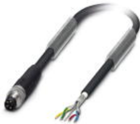
Bus system cable, INTERBUS, INTERBUS, 4-position, PUR halogen-free, Black RAL 9005, shielded, Plug straight M8, on Free cable end, Cable length: 2 m
