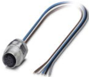
Sensor/Actuator flush-type socket, 5-pos., M12, A-coded, front/screw mounting with Pg9 thread, can be positioned, with 0.5 m TPE litz wire, 5 x 0.34 mm 2
