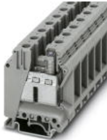
Feed-through terminal block, Connection method: Screw connection, Number of positions: 1, Cross section: 16 mm 2 - 50 mm 2 , AWG: 6 - 1/0, Width: 20 mm, Color: gray, Mounting type: NS 35/15, NS 32, NS 35/15-2,3
