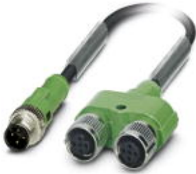
Sensor/Actuator cable, 4-position, PUR halogen-free, Black-gray RAL 7021, Plug straight M12 SPEEDCON, A-coded, on Socket straight M12 SPEEDCON, A-coded and Socket straight M12 SPEEDCON, A-coded, Cable length: 0.6 m
