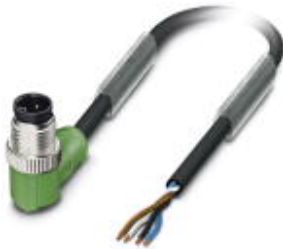
Sensor/Actuator cable, 4-position, PUR halogen-free, Black-gray RAL 7021, Plug angled M12, A-coded, on Free cable end, Cable length: 3 m
