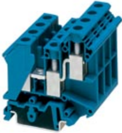
1-level terminal block with double connection on one side, cross section: 0.5 - 10 mm 2 , AWG: 24 - 6, width: 10.2 mm, color: blue
