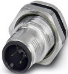
Sensor/actuator flush-type plug, 4-pos., M12 SPEEDCON, A-coded, rear/screw mounting with M16 thread, with straight solder connection
