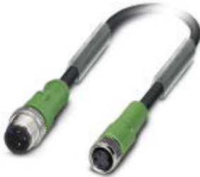
Sensor/Actuator cable, 3-position, PUR halogen-free, Black-gray RAL 7021, Plug straight M12, A-coded, on Socket straight M8, Cable length: 0.3 m
