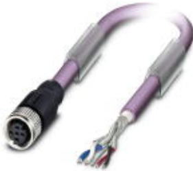
Bus system cable, CANopen ® , DeviceNet ™ , CANopen ® /DeviceNet ™ , 5-position, PUR halogen-free, Violet, RAL 4001, shielded, Free cable end, on Socket straight M12, A-coded, Cable length: 10 m
