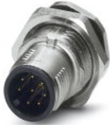
Sensor/actuator flush-type plug, 8-pos. with shield contact, M12 SPEEDCON, rear/screw mounting with M16 thread, with straight solder connection
