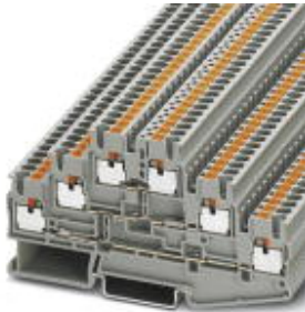
Multi-level terminal block, Cross section: 0.14 mm 2 - 4 mm 2 , AWG: 26 - 12, Connection type: Push-in connection, Width: 5.2 mm, Color: gray, Mounting type: NS 35/7,5, NS 35/15
