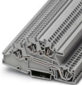
Installation level terminal block, Spring-cage connection, Cross section: 0.08 mm 2 - 4 mm 2 , AWG: 28 - 12, Width: 5.2 mm, Color: gray, Mounting type: NS 35/7,5, NS 35/15
