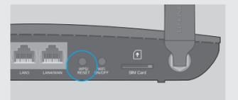
WPS/RESET Button - Press and hold until the Power LED starts flashing.
