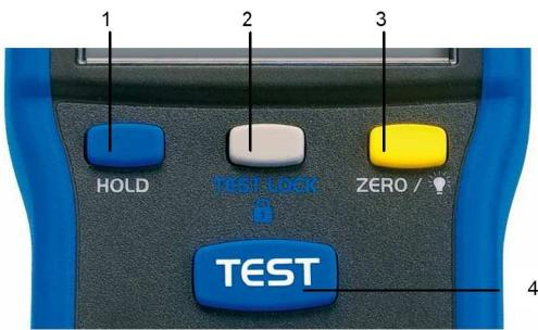
Figure 3: the keys on the keypad
