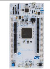
Top view of a NUCLEO-L4XXZY board without Ethernet peripheral.
