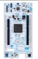
Top view of a NUCLEO-FXXXZY board without Ethernet peripheral.
