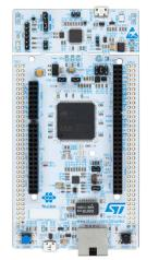
Top view of a NUCLEO-FXXXZY board with Ethernet peripheral.
